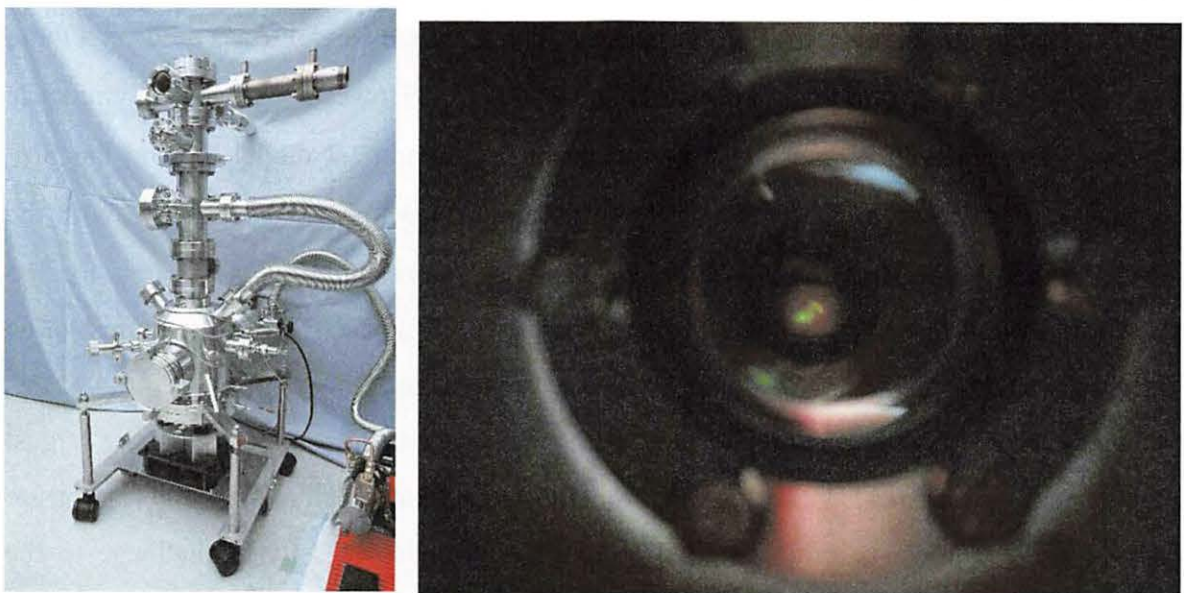
Figure 3. The left picture shows the developed thermal ionizer, and right picture shows the Rb beam profile which was observed from the thermal ionizer for the first time.
