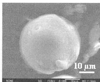
Figure 2. SEM image of the surface of (Calix[4] + Dodecanol)/SiO 2 -P.
