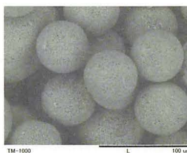
b) Microscopic image of iso heptyl -BTP resins (magnification: 800 ).
