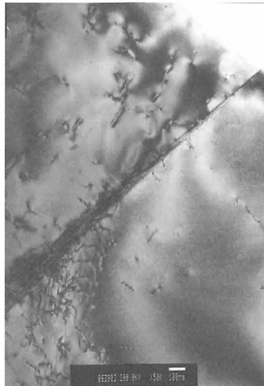
Figure 9. The microstructure of the He implanted 316FR steel up to about 1 appm.
