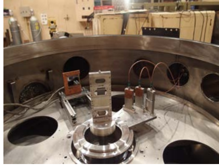
Figure 1. Inside of scattering chamber. The natural carbon foil target is placed at the center of the chamber. Three SDs are located at the right side of the chamber.
