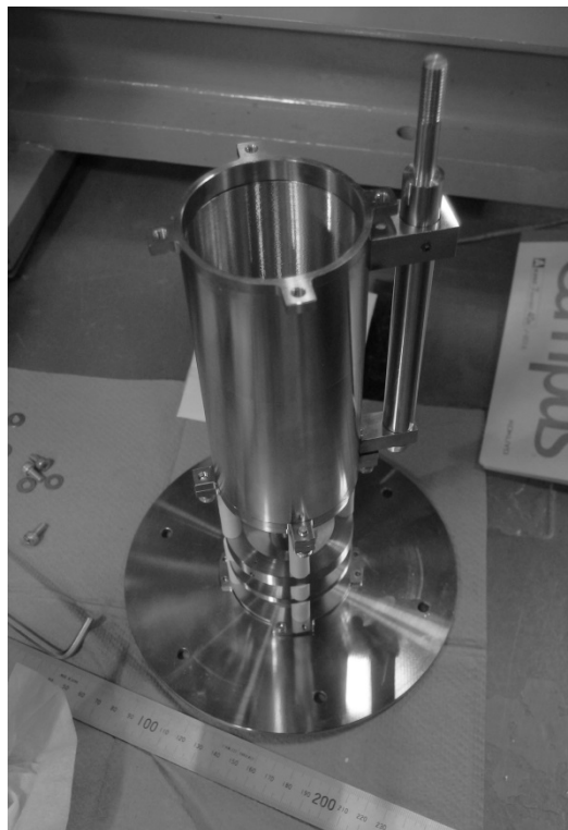
Figure 4. Picture of tetrode extraction system.
