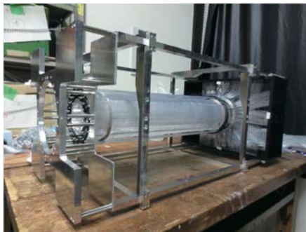
Figure 2. Photograph of the CFT prototype. Three layers are combined together. The readout MPPCs are mounted at the black frame at the downstream.
